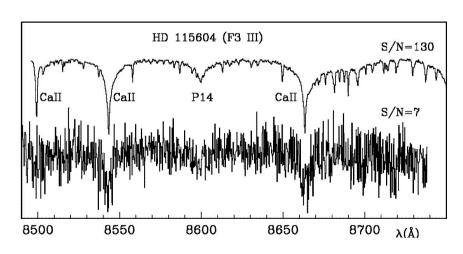
RVS spectra of F3 giant (V=16) S/N = 7 (single measurement) S/N = 130 (summed over mission)
